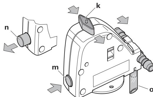
k = rotary switch position "Operation"
