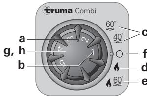
a = Rotary switch for room temperature (1 – 5)
